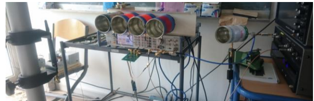
Fig. 10 Experiment setup for WiFi based passive sensor detection.
