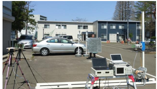
Fig. 6 Experiment setup for passive bistatic SAR imaging.
