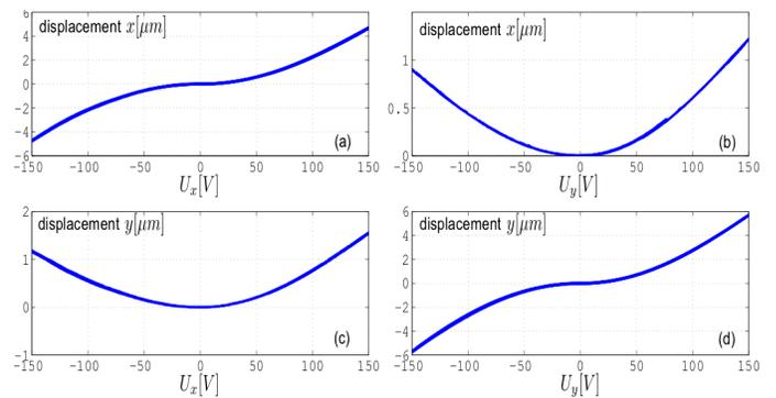
Fig. 7. Output displacement ( $x$  and  $y$ ) versus input voltages ( $U_x$  and  $U_y$ ).
