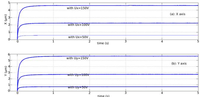
Fig. 8. Step responses along  $x$  and  $y$  axis for different input voltages.
