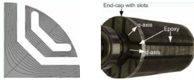
Fig.7 Epoxy-filled rotor [14]: (a) design structure (b) rotor manufactured
