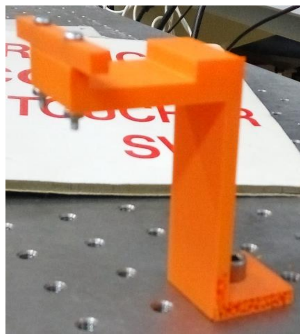
Fig. 5 Support designed with AutoCAD and 3D printed.
