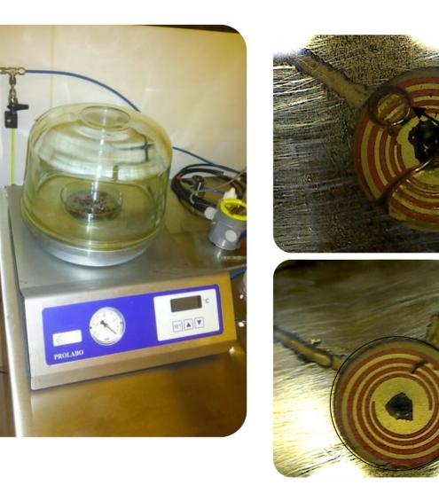
Air bubble in cavity when pressure in chamber is 800 mbar
