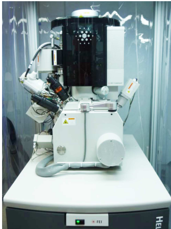
Figure 4.6: Photograph of the SEM/FIB dual-beam system (Helios Nanolab 600i, FEI) available at FEMTO-ST Institute. It is the workhorse for both structuring and characterizing HPAs.
