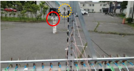
Fig. 5. Experiment with two trihedral corner reflectors as targets.
