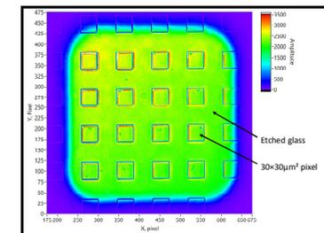
Figure 4. Transmission at 770 nm of a pixelated filters.
