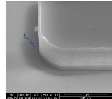
Figure 3. SEM cross section of etched Nb<sub>2</sub>O<sub>5</sub>/SiO<sub>2</sub> multilayer.
