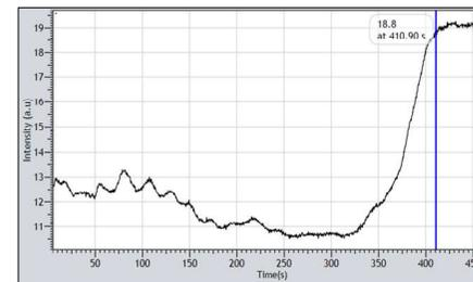
Figure 2. EPD detection of etching of the multilayers Nb<sub>2</sub>O<sub>5</sub>/SiO<sub>2</sub>.
