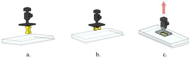
**Fig. 3** Different build orientations: a) longitudinal, b) transverse, c) normal.
