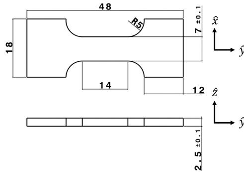
**Fig. 2** Specimen dimensions (mm).
