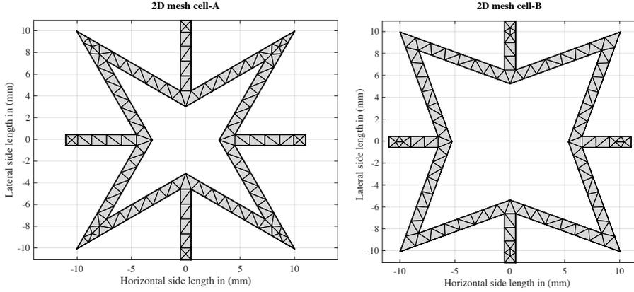
Figure 2: 2D mesh of cell-A and cell-B
