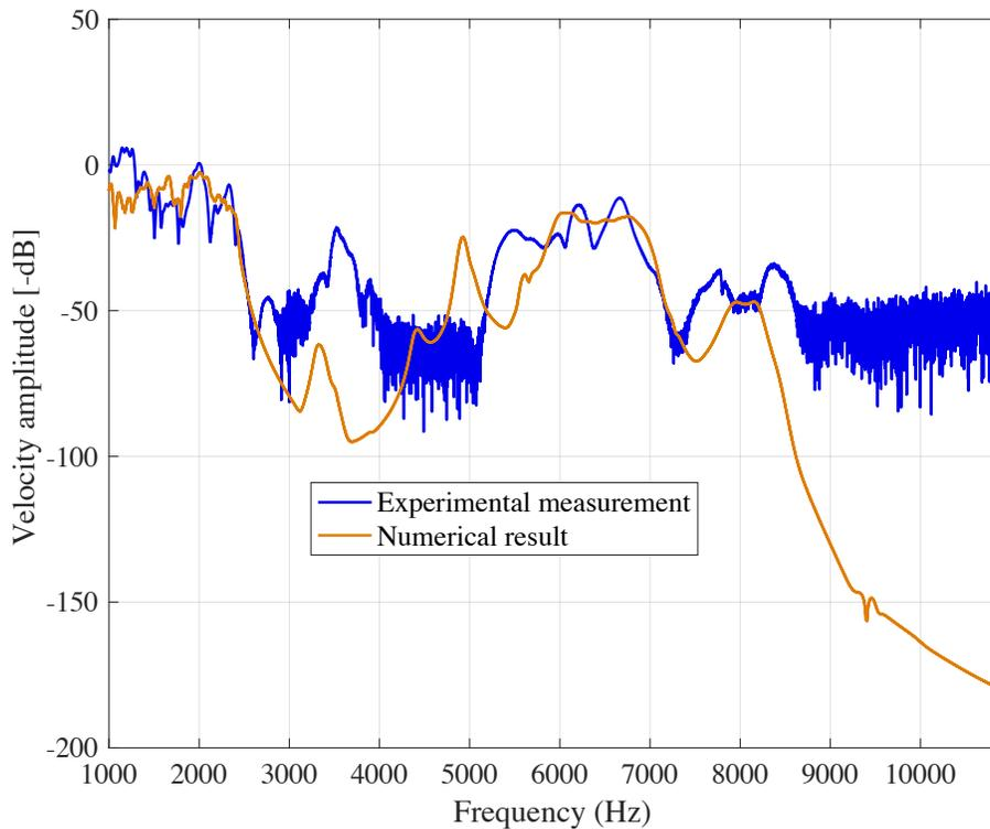
Figure 22: Comparison of numerical and experimental FRFs
