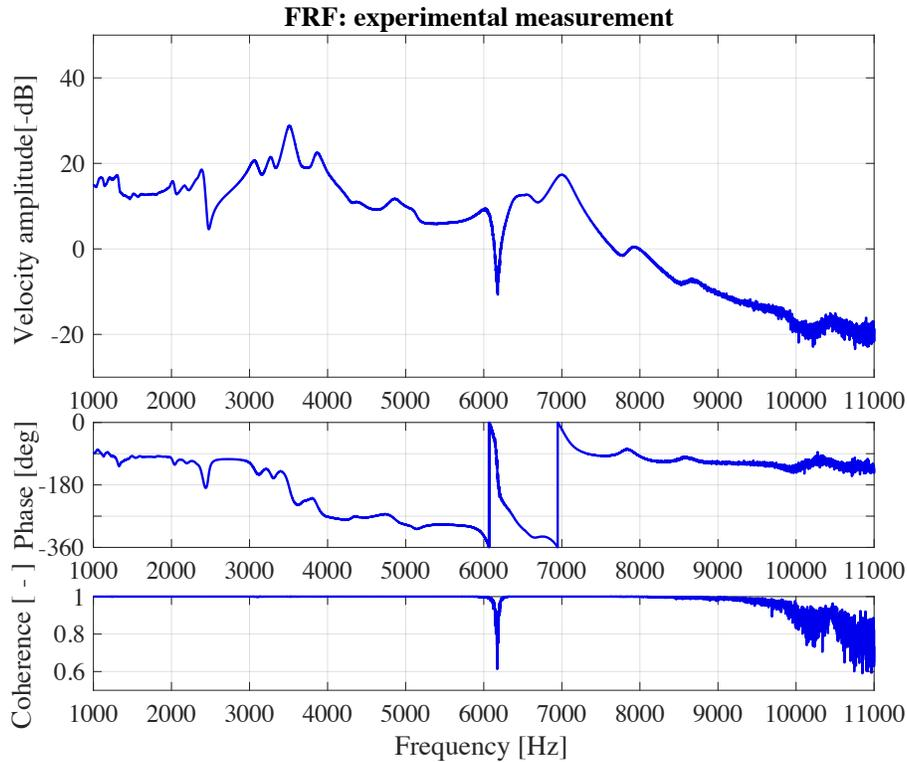
Figure 13: Velocity response measured in the input point
