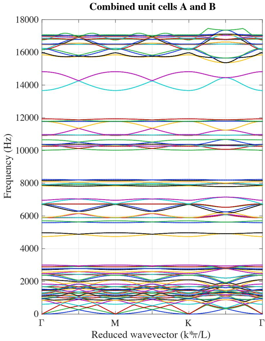
Figure 9: Band diagram of combined A-B lattice
