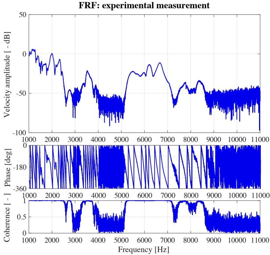
Figure 14: Velocity response measured in the output point
