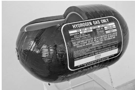
Fig. 3. CGH2 tank produced by Korean manufacturer ILJIN [3].
