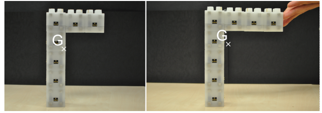
Figure 7: Example for a stable and an unstable configuration for the T-shape stability test
