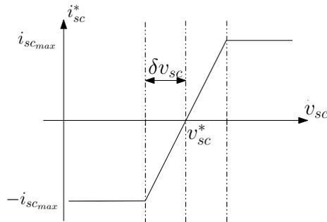
**Figure 9.** Definition of the SCs current according to the SCs voltage for controller 2.
