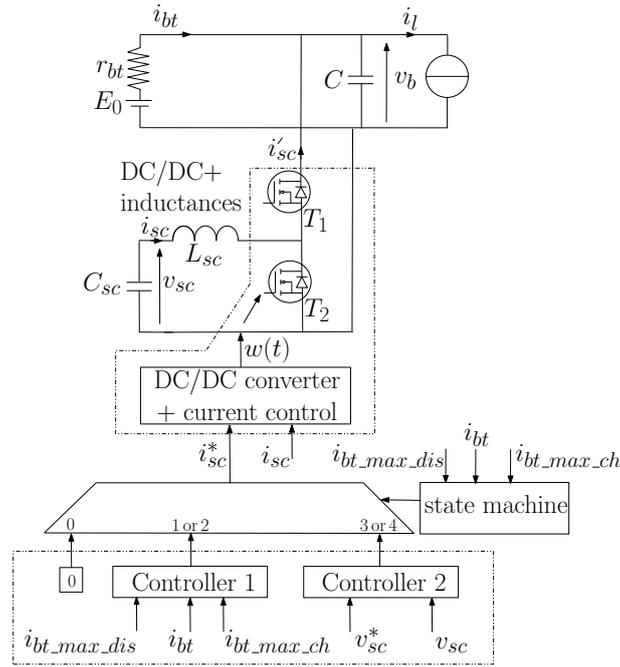
**Figure 5.** Controllers of the charge depleting mode with SoC recovering of the SCs.
