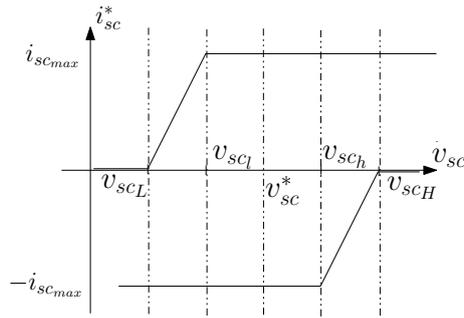
**Figure 8.** Definition of the maximum SCs current ( $i_{sc_{max}}$ ) according to the SCs voltage for controller 1.
