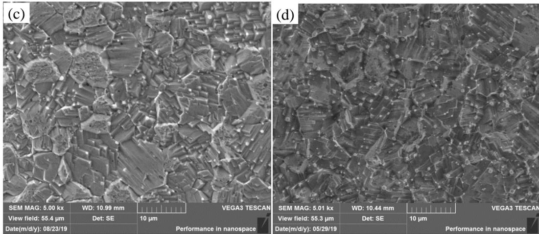
Fig. 2. Microstructure of alloys: (a) Pure W; (b) W-0.25wt%Zr(Y)O<sub>2</sub>; (c) W-0.5wt%Zr(Y)O<sub>2</sub>; (d) W-0.75wt%Zr(Y)O<sub>2</sub>.
