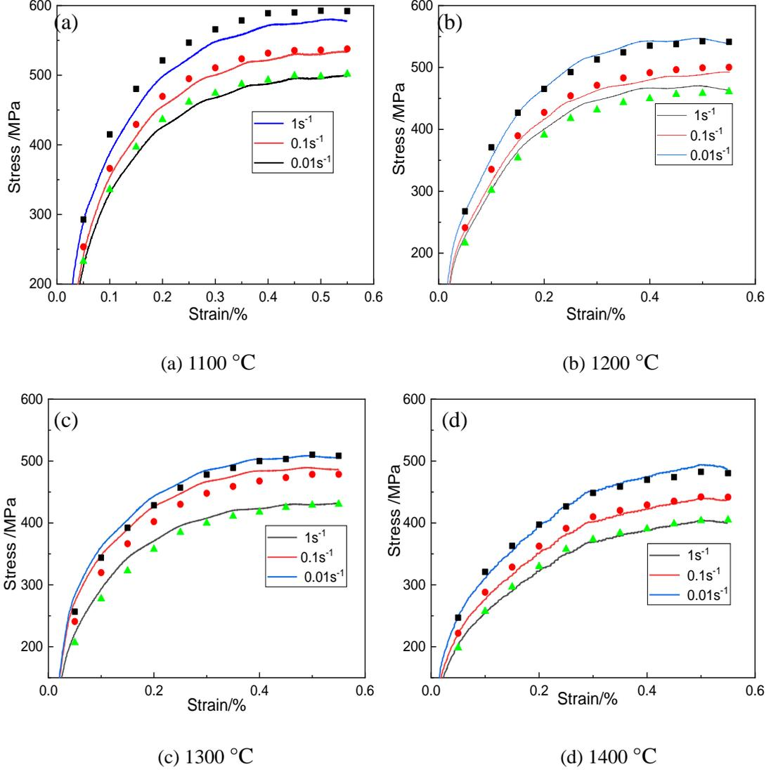
Fig. 7. True stress-strain curves of the W-0.25wt%Zr(Y)O<sub>2</sub> alloy under different deformation conditions: (a) 1100 °C; (b) 1200 °C; (c) 1300 °C; (d) 1400 °C.
