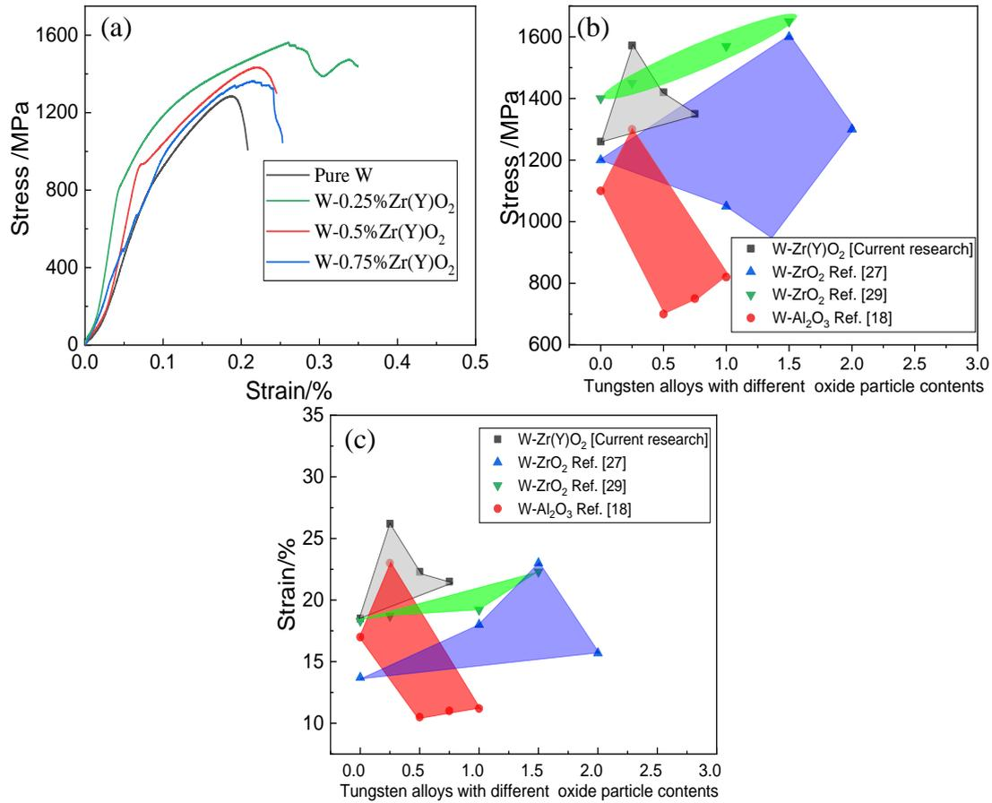
Fig. 5. (a) Compressive stress-strain curves of W alloys with different Zr(Y)O<sub>2</sub> contents; (b) Compressive strength and (c) Fracture strain of W-Zr(Y)O<sub>2</sub> alloy in comparison with available literature datas.
