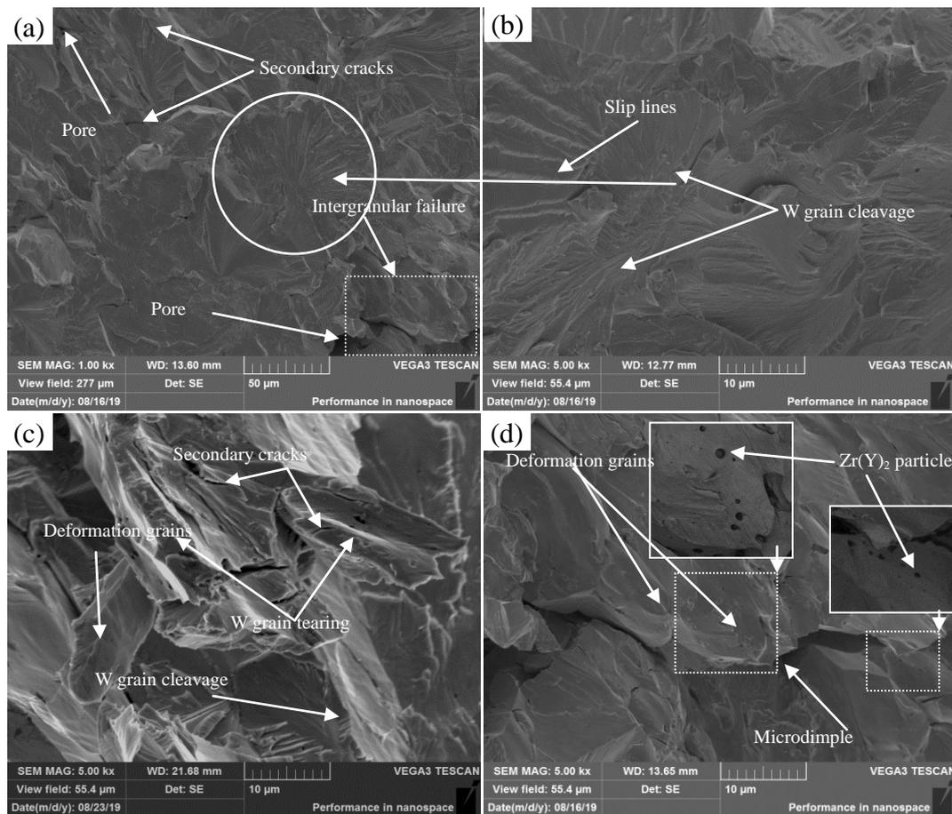
Fig. 6. Fracture surface of W-0.25%Zr(Y)O<sub>2</sub> alloy
