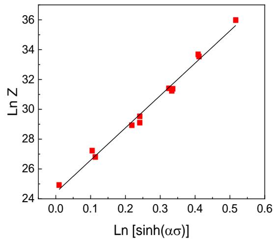
Fig. 10 Relationship between  $\ln[\sinh(\alpha\sigma)]$  and  $\ln Z$ .
