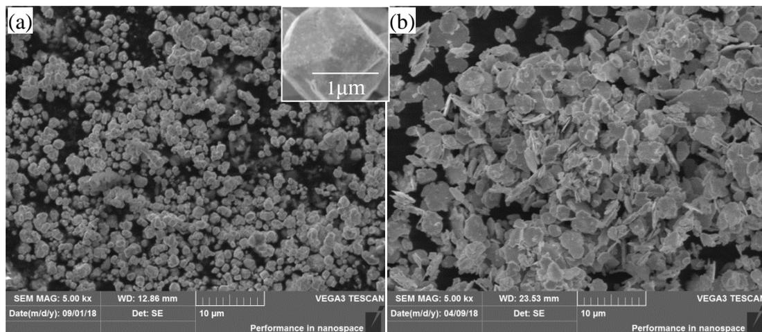
Fig. 1. SEM images of W-0.75wt%Zr(Y)O<sub>2</sub> powders prepared through different methods: (a) Hydrothermal method; (b) Hydrothermal method, followed by mechanical alloying.
