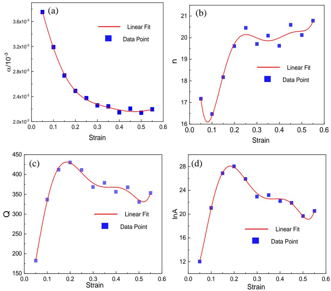
Fig. 11. Relationship between the strain and material constants: (a)  $\alpha$ ; (b)  $n$ ; (c)  $Q$ ; (d)  $\ln A$ .
