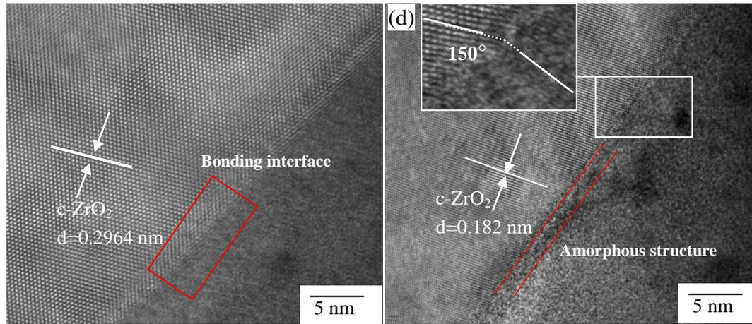
Fig. 4(a, b) TEM images of tungsten alloy showing Zr(Y)O<sub>2</sub> particles; (c) HREM image of tungsten alloy; (d) HREM image of Zr(Y)O<sub>2</sub>/W interface
