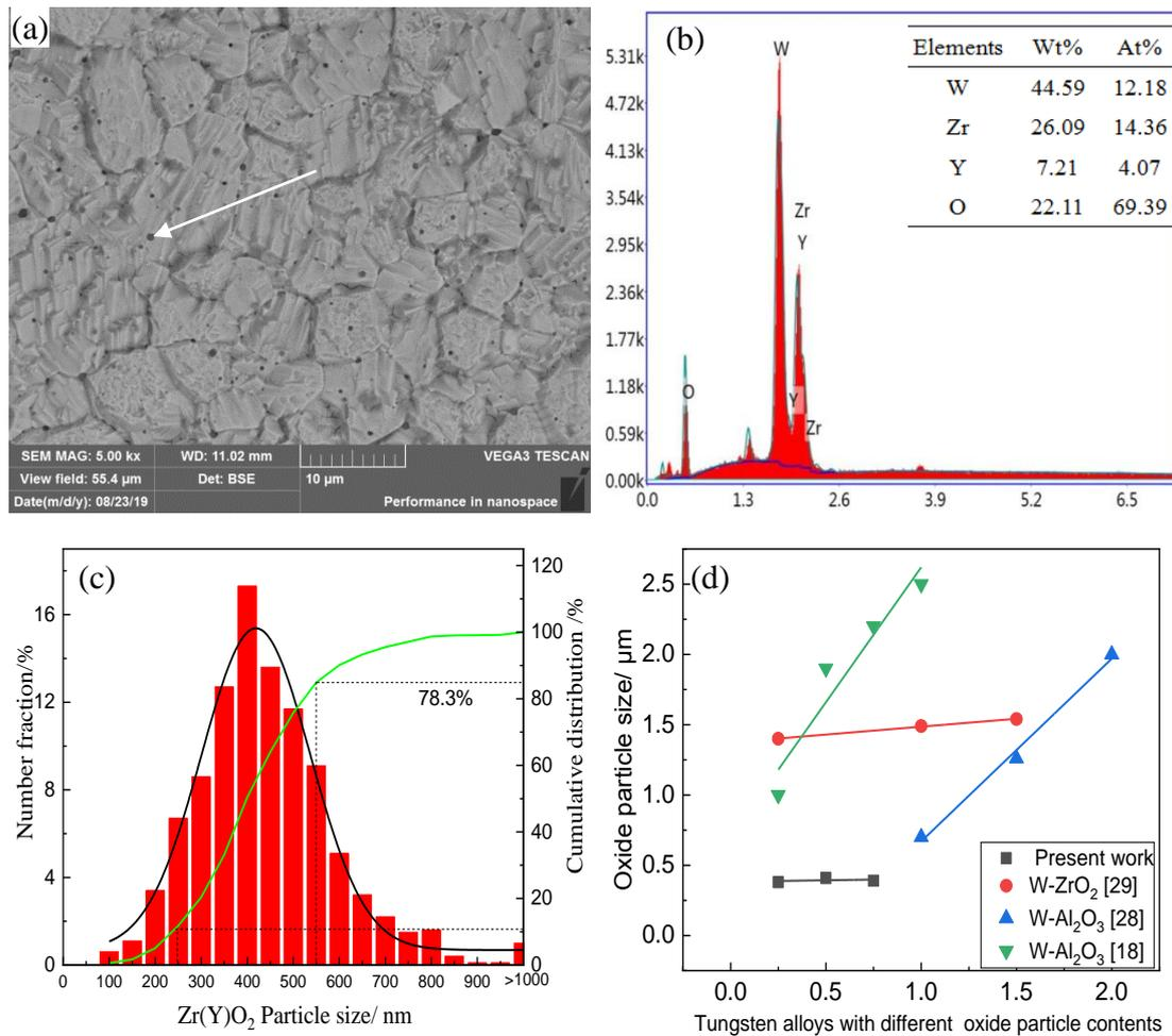
Fig. 3. (a) BSE image of tungsten alloys with 0.5wt%Zr(Y)O<sub>2</sub> alloy; (b) EDS spectrum on the white arrow A in Fig. 3a; (c) Particle size distribution of Zr(Y)O<sub>2</sub> in W-0.5wt%Zr(Y)O<sub>2</sub> alloy and (d) Particle size VS W alloys reinforced different
