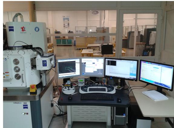
Fig. 3 Carl Zeiss Auriga SEM used in experiments.
