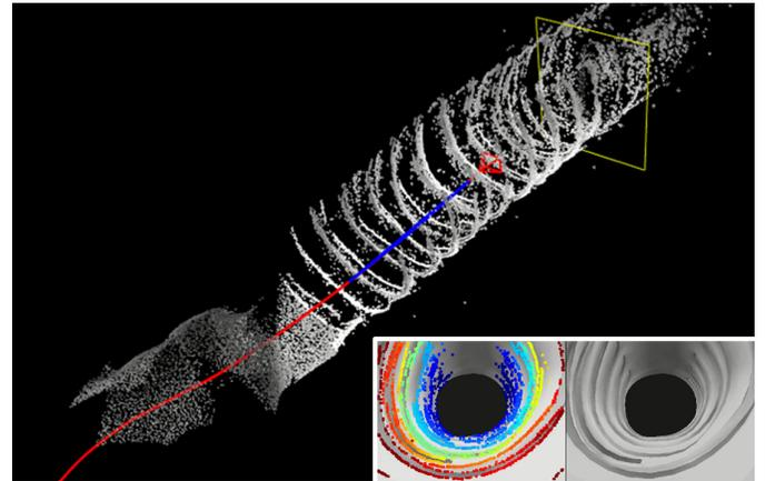
Fig. 3. *Top*: reconstructed 3-D shape of the environment given by the DSO-SLAM algorithm, with the red lines showing the camera trajectory. *Bottom*: frame obtained by the virtual camera during deployment, with and without the detected keypoints.
