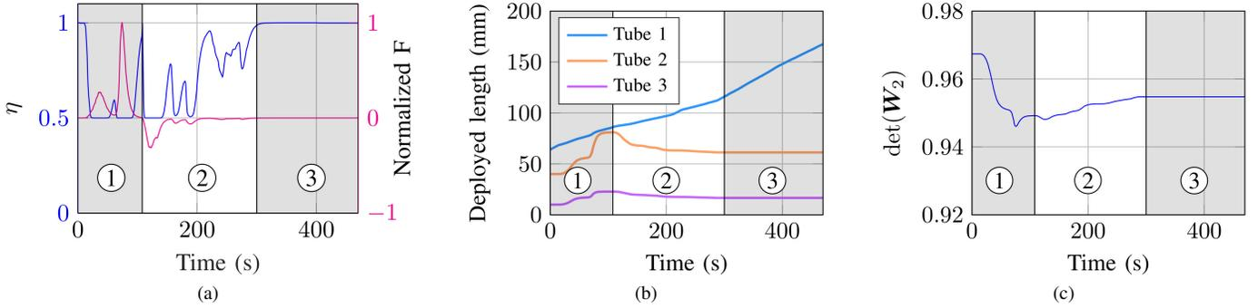
Fig. 5. (a) normalized repulsive force  $F$  (filtered) and  $\eta$ , (b) deployed tube lengths, and (c) stability of the CTR over time, with the deployment steps identified and labeled, during deployment in the trachea.
