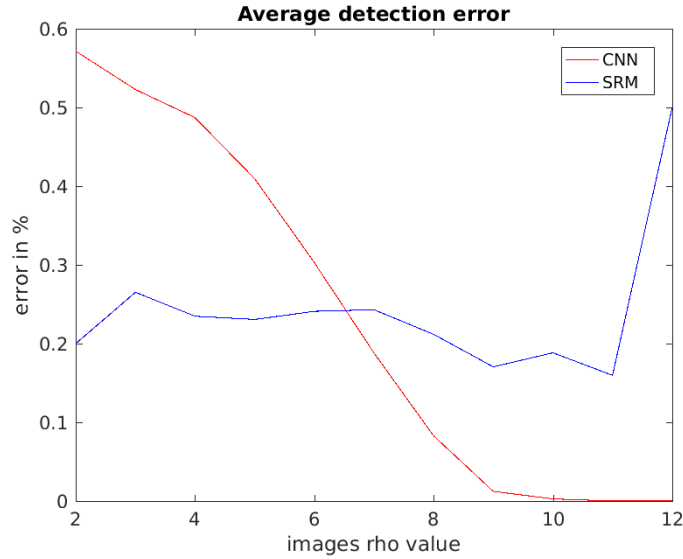
Figure 4.10: Average detection error of CNN-based and SRM+EC steganalyzers for MiPOD 0.4 bpp w.r.t \bar{\rho}_U .
