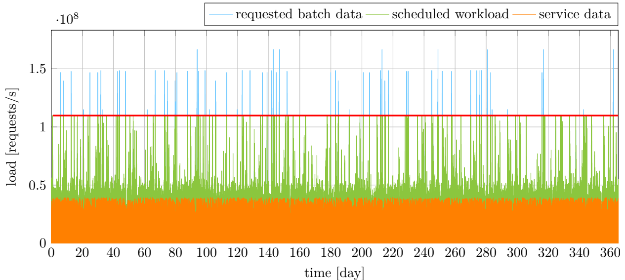
Figure 2: Example of the load (expressed as a histogram in number of requests per seconds) over time (in hours) which is executed after the IT sizing. The requests for services are in orange, the ones for batches in blue. It results in the green processed requests using 1098 servers considering one year discretized into K = 8760 time slots of one hour and a flexibility of 3 hours.
