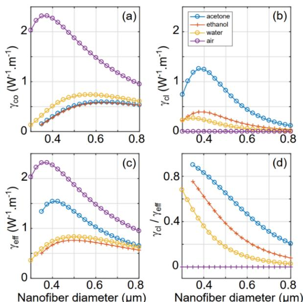
Figure 1. Evolution in function of the nanofiber diameter and for different surrounding media of (a) the nonlinear parameter contribution of the silica core  $\gamma_{co}$  (b) the nonlinear parameter contribution of the cladding  $\gamma_{cl}$ , (c) the whole effective nonlinear parameter  $\gamma_{eff}$ , and (d) the  $\gamma_{cl}/\gamma_{eff}$  ratio. Wavelength  $\lambda = 532\text{nm}$ .
