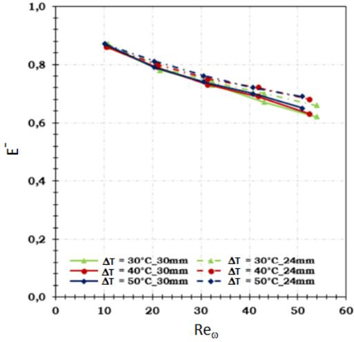
Figure 11: Variation of the thermal efficiency of the regenerator  $E^-$  during hot-blow with piston stroke  $C = 30$  mm, porosity  $\epsilon = 0.90$ , as a function of the frequency Reynolds number  $Re_\omega$  and temperature differences  $\Delta T = 30^\circ C, 40^\circ C$  and  $50^\circ C$
