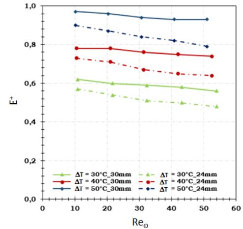
Figure 10: Variation of the thermal efficiency of the regenerator  $E^+$  during cold-blow with piston stroke  $C = 30$  mm, porosity  $\epsilon = 0.9$ , as a function of the frequency Reynolds number  $Re_\omega$  and temperature differences  $\Delta T = 30^\circ C$ ,  $40^\circ C$  and  $50^\circ C$
