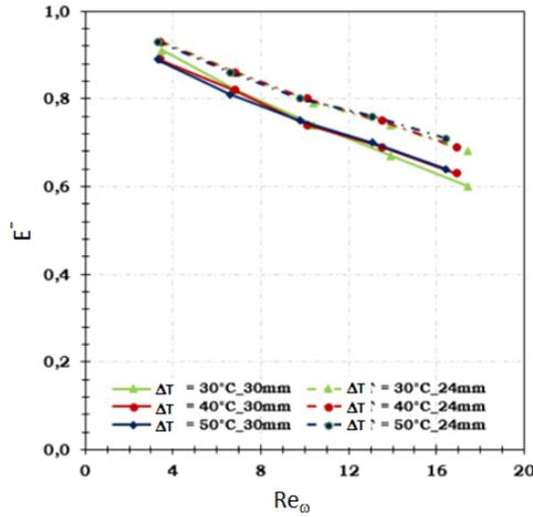
Figure 9: Variation of the thermal efficiency of the regenerator  $E^-$  during hold-blow with piston stroke  $C = 30$  mm, porosity  $\epsilon = 0.8$ , as a function of the frequency Reynolds number  $Re_\omega$  and temperature differences  $\Delta T = 30^\circ C$ ,  $40^\circ C$  and  $50^\circ C$
