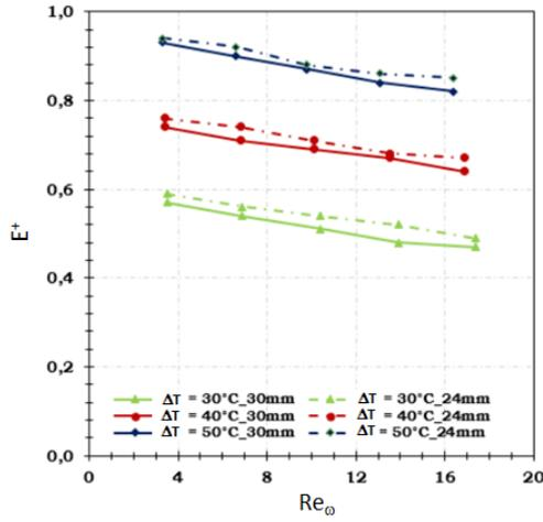
Figure 8: Variation of the thermal efficiency of the regenerator  $E^+$  during cold-blow with piston stroke  $C = 24$  mm, porosity  $\epsilon = 0.8$ , as a function of the frequency Reynolds number  $Re_\omega$  and temperature differences  $\Delta T = 30^\circ C$ ,  $40^\circ C$  and  $50^\circ C$
