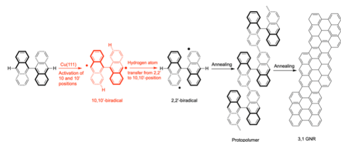
Scheme 2: Completed reaction mechanism for the growth of (3,1) GNR induced by a two-step annealing of BA molecules on a Cu(111) surface. The formation of 10,10'-biradical (in red), followed by radical transposition, is added as initial step.
