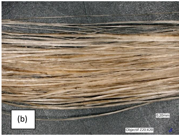
Figure 3: Example of non-retted fibres (a) and retted fibres (b)
