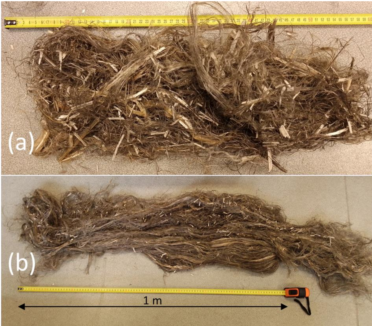
Figure 2: Scutching tows: (a) mixture of shives, short and average length fibres; (b) Shives and long line fibres
