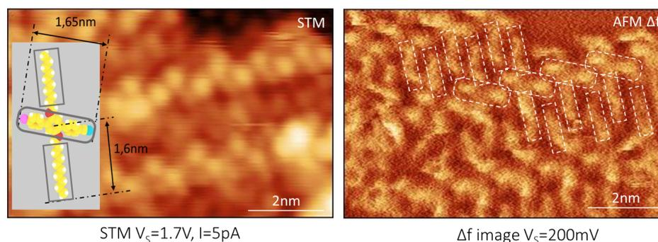
Figure : STM (left) and nc-AFM  $\Delta f$  image (right) of the investigated molecular array (see text), using an oscillating probe with total oscillation amplitude  $A_{pp}=100pm$ .
