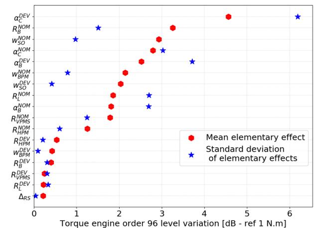
Fig. 7. Torque engine order 96 sensitivity to parameter variations.
