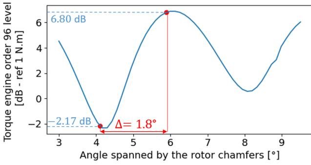
**Fig. 9.** Effect of the parameter  $\alpha_c$  on the torque engine order 96 level, for the design used to calculate its largest elementary effect due to deviations.
