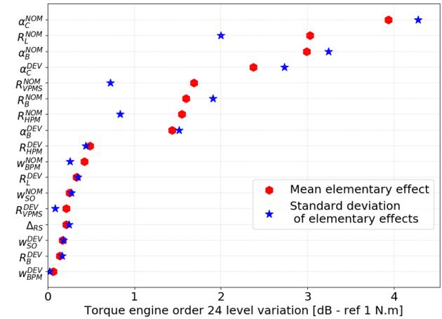
Fig. 5. Torque engine order 24 sensitivity to parameter variations.
