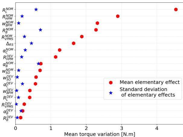
Fig. 4. Mean torque sensitivity to parameter variations.
