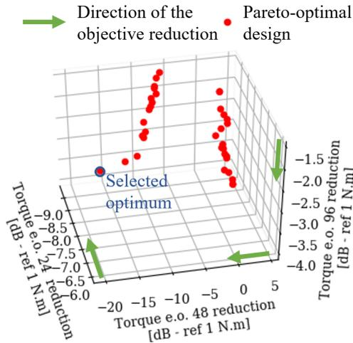
**Fig. 10.** Values of the objectives of the designs belonging to the estimated Pareto front for the classical multiobjective optimization aiming at minimizing the torque engine orders 24, 48 and 96 – first overview
