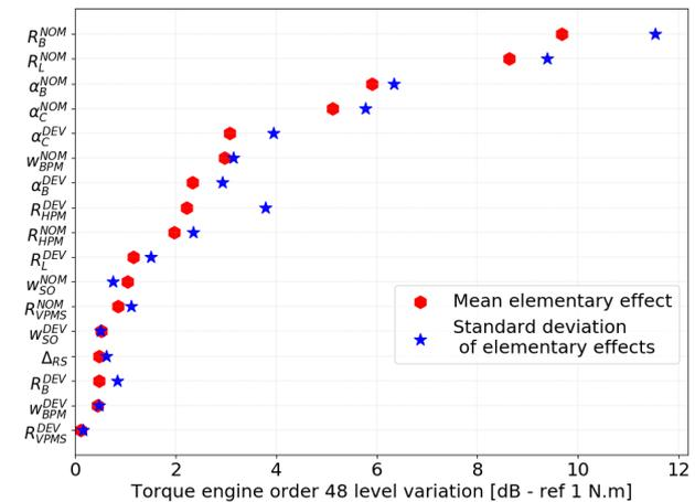
Fig. 6. Torque engine order 48 sensitivity to parameter variations.
