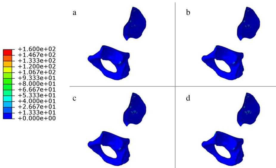
**Figure 7.** Stress field in the cortical bone for the screw pretension force of 100 N (a), 200 N (b), 300 N (c) and 400 N (d). Von Mises equivalent stress, MPa.
