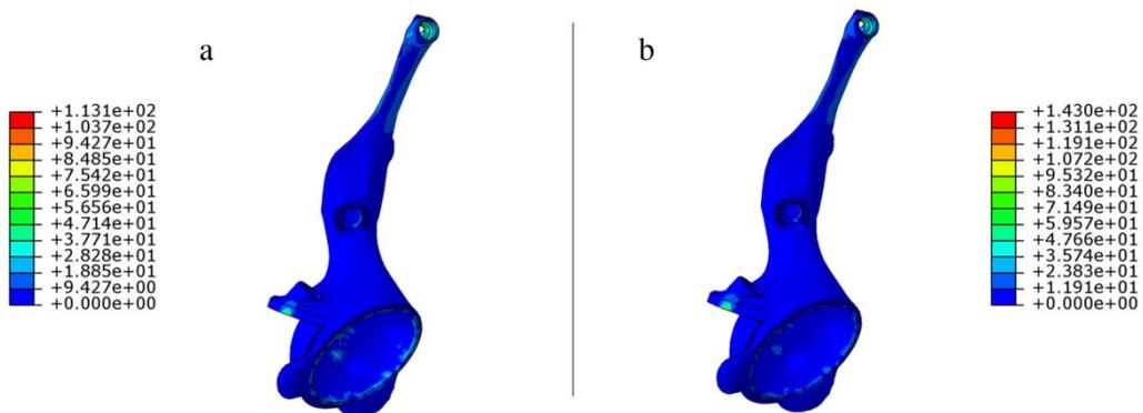
**Figure 10.** Stress field in the customized implant for the screw pretension force of 200 N (a) and 300 N (b). Von Mises equivalent stress, MPa.
