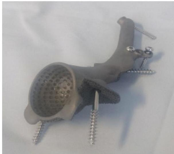
**Figure 3.** Additively manufactured customized implant [14].
