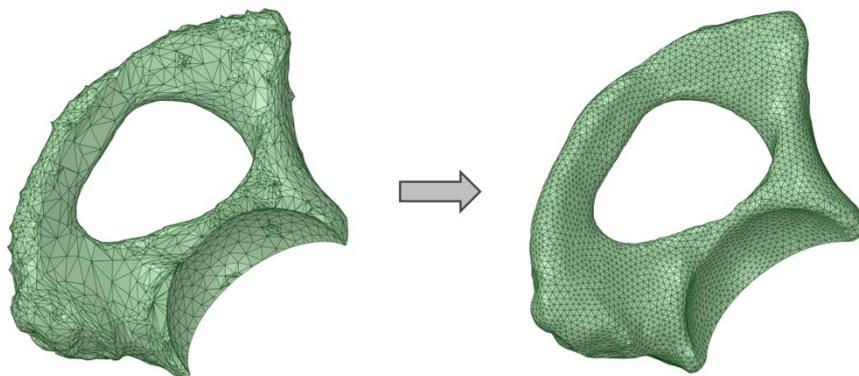
**Figure 4.** Results of the mesh processing from the geometrical triangular mesh to the finite element mesh.
