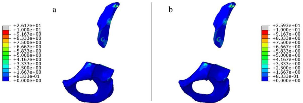
**Figure 8.** Stress field in the spongy bone for the screw pretension force of 200 N (a) and 300 N (b). Von Mises equivalent stress, MPa.
