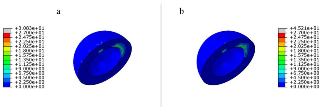
**Figure 12.** Stress field in the acetabular cup for the screw pretension force of 200 N (a) and 300 N (b). Von Mises equivalent stress, MPa.
