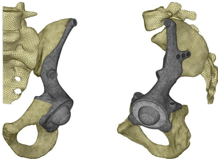
**Figure 5.** Finite element mesh of the pelvic, implant, acetabular cup and femur head.
