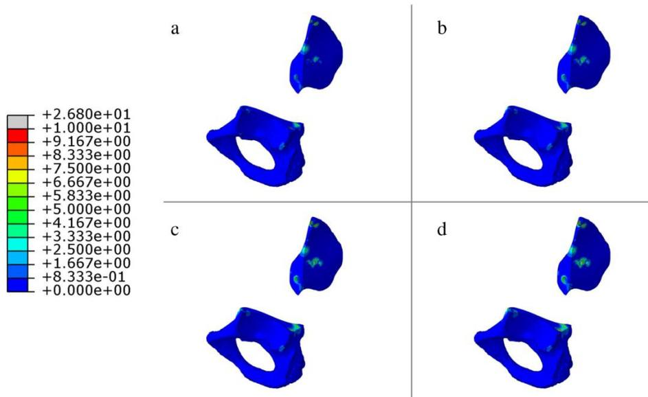
**Figure 6.** Stress field in the spongy bone for the screw pretension force of 100 N (a), 200 N (b), 300 N (c) and 400 N (d). Von Mises equivalent stress, MPa.
