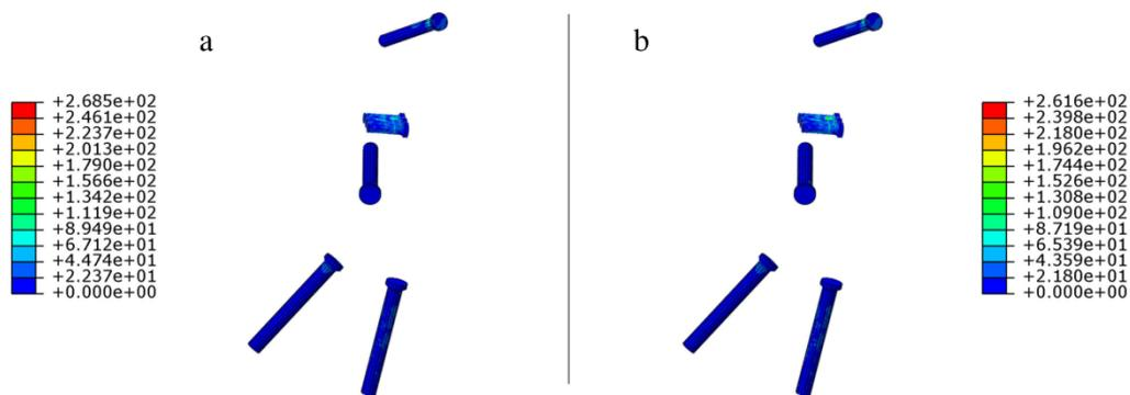
**Figure 11.** Stress field in the screws for the screw pretension force of 200 N (a) and 300 N (b). Von Mises equivalent stress, MPa.
