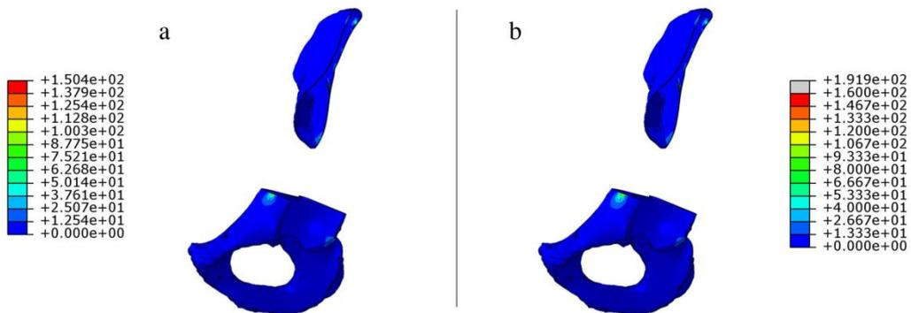
**Figure 9.** Stress field in the cortical bone for the screw pretension force of 200 N (a) and 300 N (b). Von Mises equivalent stress, MPa.
