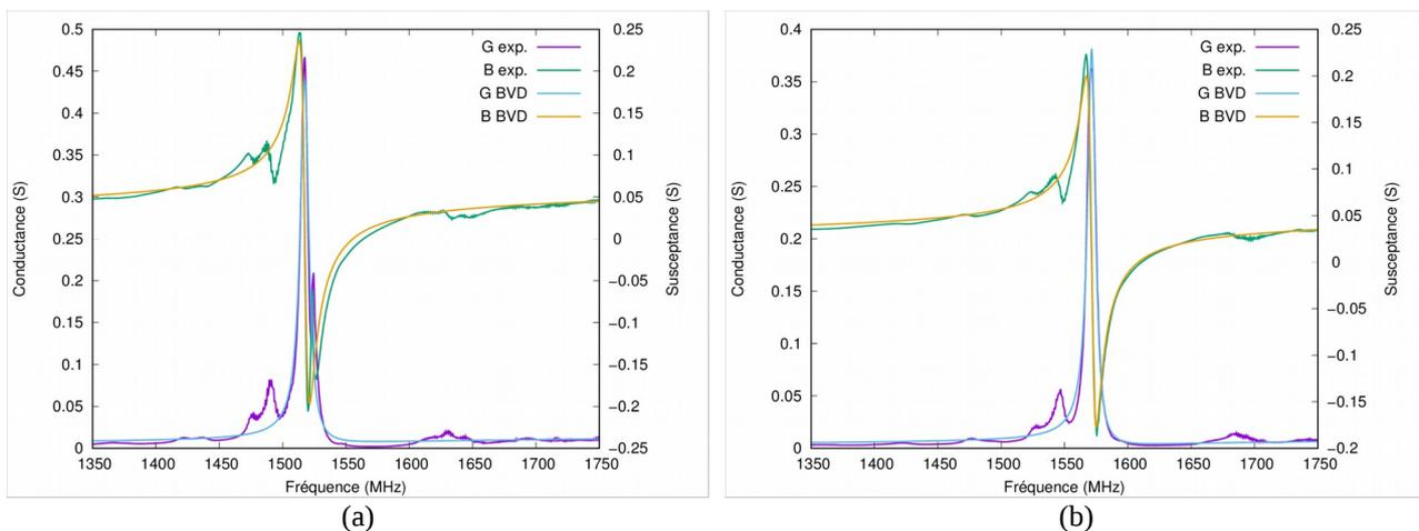
Fig. 5. Typical measurements of parallel and series resonators prior to the final design of the GPS filter, characterization of the main resonator and mode properties using a Butterworth – Van Dyke equivalent circuit and mixed matrix model (a) parallel resonator (b) series resonator
