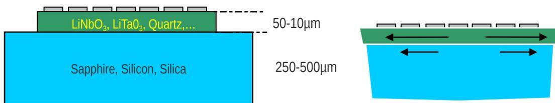
Fig. 1. General principle of a composite wafer combining a low TCE substrate impeding a top piezoelectric plate to thermally expand, limiting its sensitivity to temperature changes
