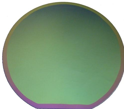
Fig. 3. Very high quality full wafer LiTaO<sub>3</sub> film transfer, 150 mm diameter wafer with SAW grade surface finishing
