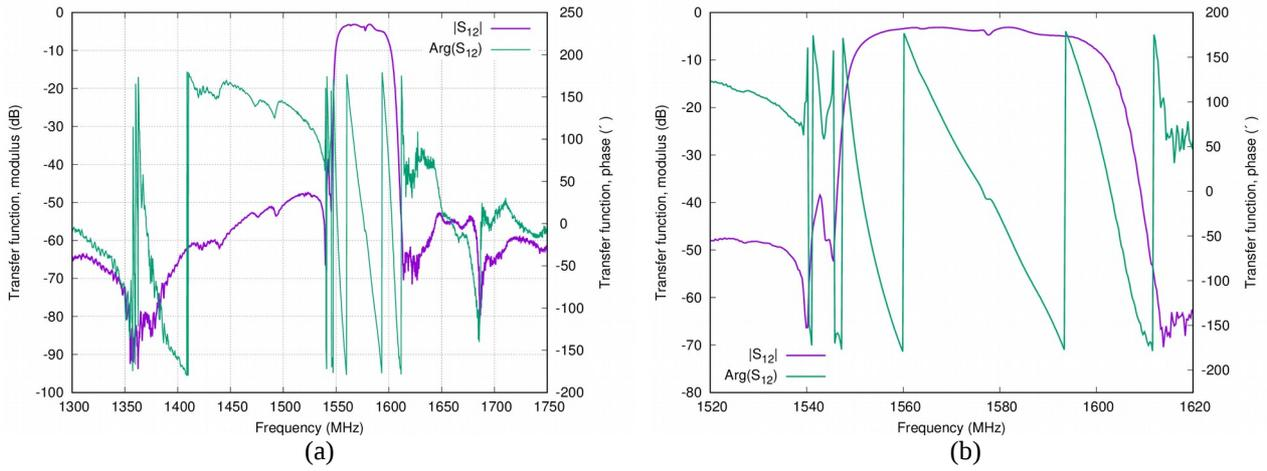
Fig. 6. Filter (a) Wide band transfer function  $|S_{12}|$  (b) Zoom on the close bandpass rejection
