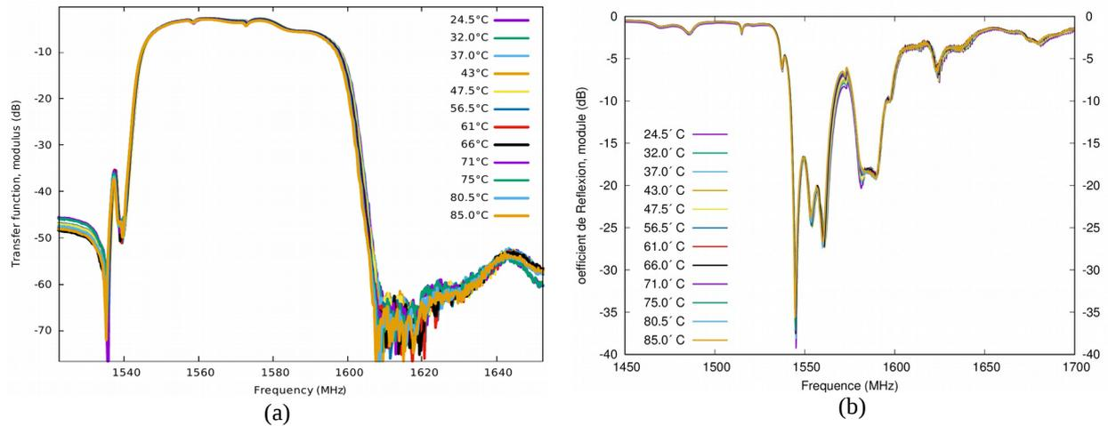
Fig. 8. Electrical response of the GPS filter built on POI at various temperature – typical temperature stability is better than  $-10 \text{ ppm.K}^{-1}$  corresponding to the upper transition band changes, the band is slightly reducing with temperature
