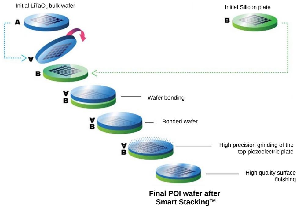
Fig. 2. Smart-Stacking<sup>®</sup> principle applied to piezoelectric-on-insulator – POI – wafers
