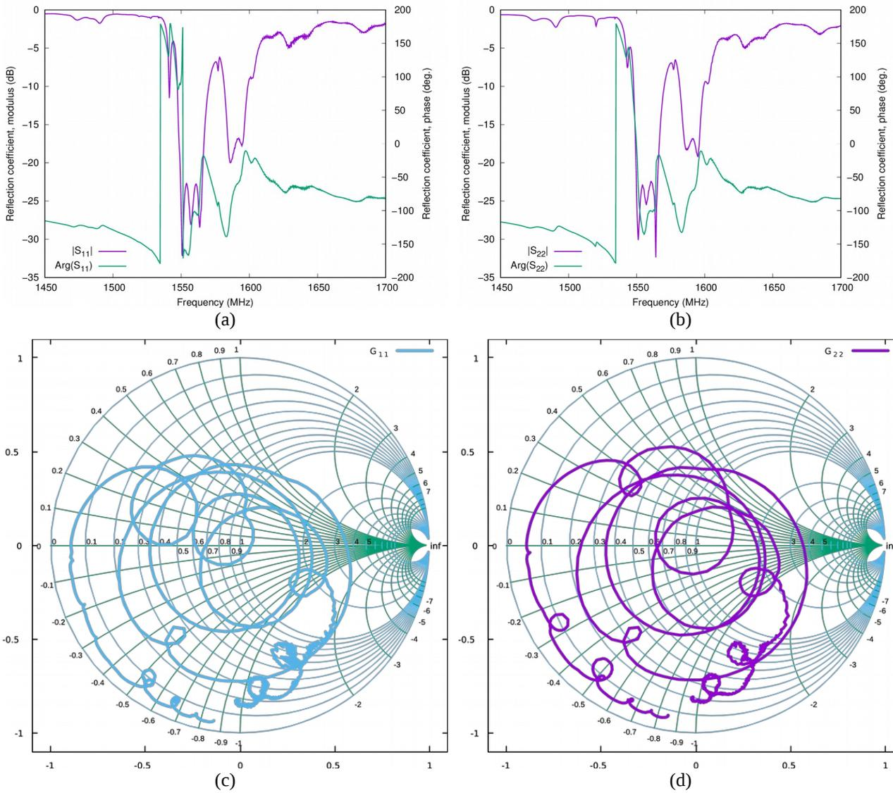
Fig. 7. Reflection parameter of the GPS filter derived from  $S_{11}$  measurements (a) Reflection coefficient – Input (b) Reflection coefficient – Output (c) Smith Chart – Input (d) Smith Chart – Output
