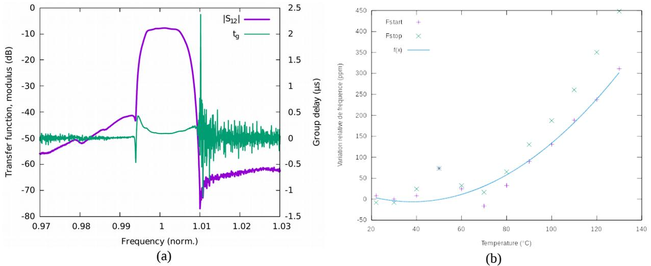
Fig. 4. 0.4% relative bandpass filter (a) Wide band transfer function  $|S_{12}|$  (b) thermal sensitivity of the filter comparable to Quartz device one but with a positive curvature opposite, proper to LiTaO<sub>3</sub>/Si substrates
