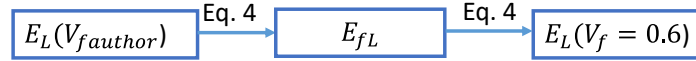
Fig. 4. Methodology used to estimate the longitudinal modulus of composites for a fiber volume fraction of 0.6
