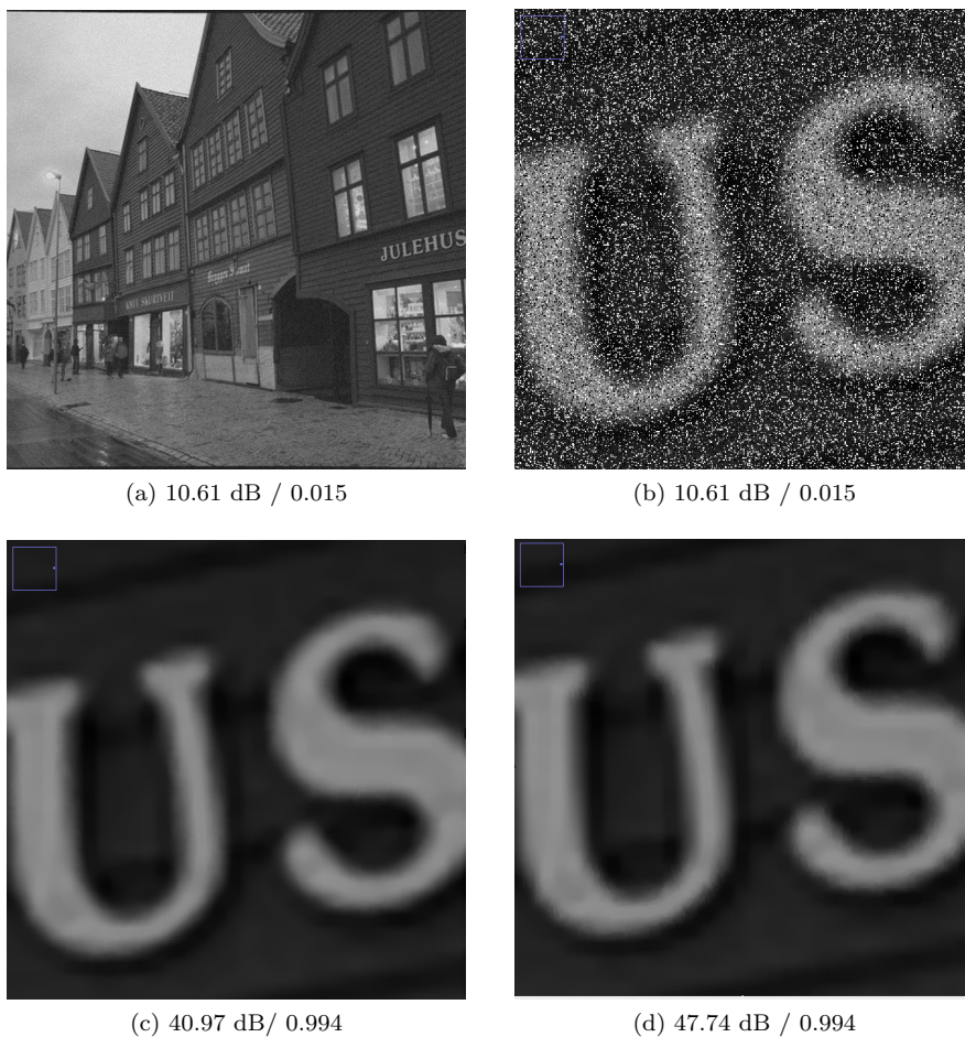
Fig. 11 Example of a 8192 \times 8192 image, corrupted by a 25% salt and pepper noise (a) and then processed by both full and separable 15 \times 15 filters. a) shows the whole image, b) focus on a 681 \times 681 pixel square around the last letters “US” on the right side. Images c) and d) are filtered using respectively the full and the separable version. For each image, results are given through PSNR(dB)/MSSIM and are computed on the whole images.
