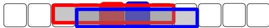
Fig. 5 Overlapping windows (framed in red and blue) of two 5 \times 1 median filters applied on adjacent pixels colored in red and blue. Filtering windows share 4 pixels.
