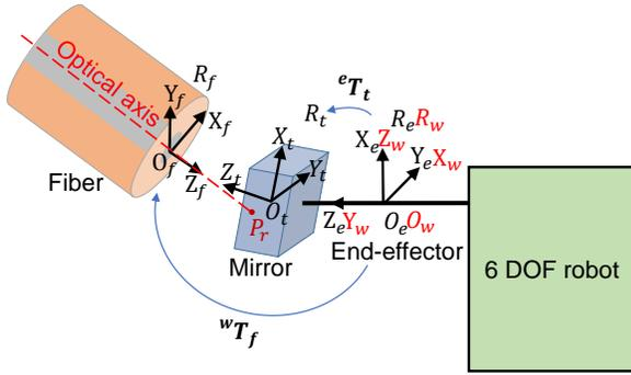
Figure 4. The robotic positioning scheme with frames assignment.
