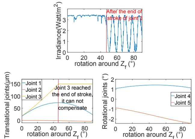
Figure 11. Rotation  $q_6$  around  $Z_f$  axes in operational coordinates when the reflection point projection is in  $P_r(141.1, 116.34)$ , after robot extrinsic and intrinsic parameters identification.
