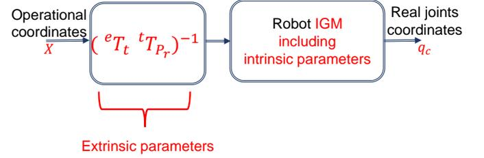
Figure 7. 6-DoF Nanopositioning robot control after full calibration.
