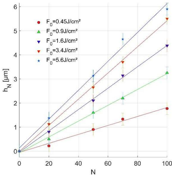
**Fig. 6.** Ablation depth  $h_N$  versus the number of pulses  $N$  for  $F_0 = 0.45, 0.9, 1.6, 3.4, 5.6 \text{ J/cm}^2$
