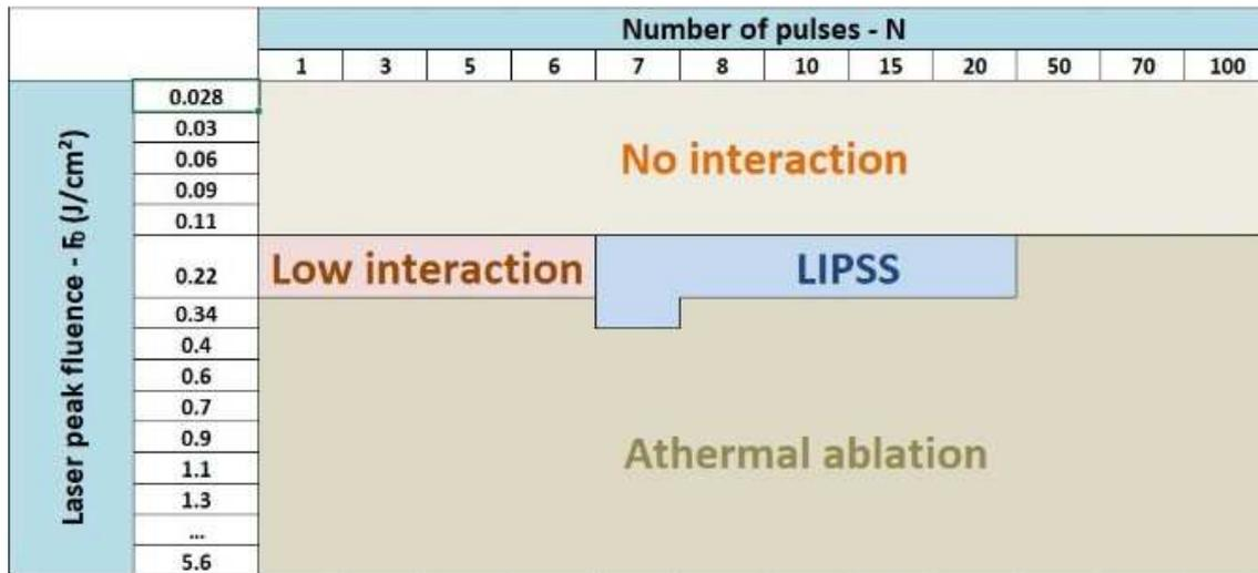
Fig. 9. Laser-matter interaction domain map for tungsten carbide.
