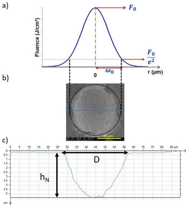
**Fig. 1. a)** Schematic of Gaussian beam profile, **b)** SEM image of crater generated on tungsten carbide material using a peak fluence  $F_0 = 2.6$  J/cm<sup>2</sup> and  $N = 100$  pulses, **c)** 2D profile of produced dimple ( $D =$  diameter,  $h_N =$  depth).
