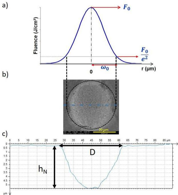
**Fig. 1. a)** Schematic of Gaussian beam profile, **b)** SEM image of crater generated on tungsten carbide material using a peak fluence  $F_0 = 2.6 \text{ J}/\text{cm}^2$  and  $N = 100$  pulses, **c)** 2D profile of produced dimple ( $D =$  diameter,  $h_N =$  depth).
