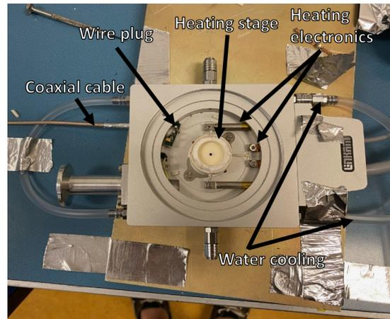
Figure 5 In-situ RF measurement set-up after modifications.
