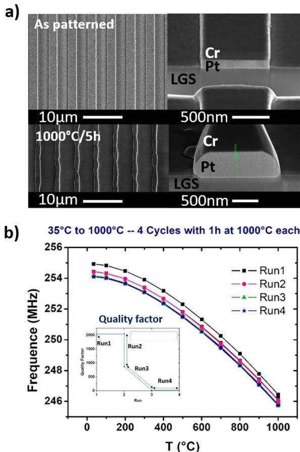
Figure 6 a) SEM micrographs of the surface and cross-section of a device as-fabricated (top) and after 5h at 1000°C (bottom), b) frequency response during 4 heating runs up to 1000°C. Inset shows the quality factor at different runs.
