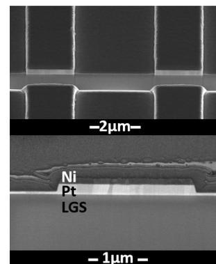
Figure 3 SEM tilted micrograph (top) and cross-section micrograph (bottom) of IDTs after Pt patterning using a nickel hard mask.
