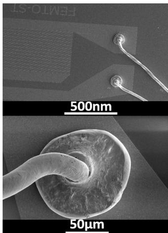
Figure 4 SEM micrographs of a wire-bonding after annealing for 3h at 800°C.
