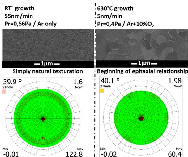
Figure 2 Comparison of the structure and grain size of Pt layers grown at room temperature with a fast recipe (left) and at 630°C with an optimized one (right).
