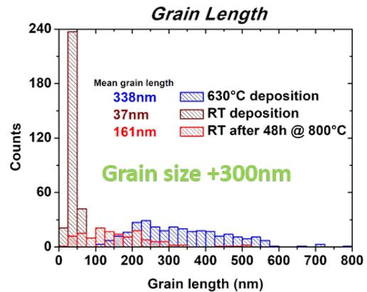
Figure 1 Distribution of the grain size of samples grown at room temperature (as deposited and annealed for 48 h at 800 °C) and film grown at 630 °C.
