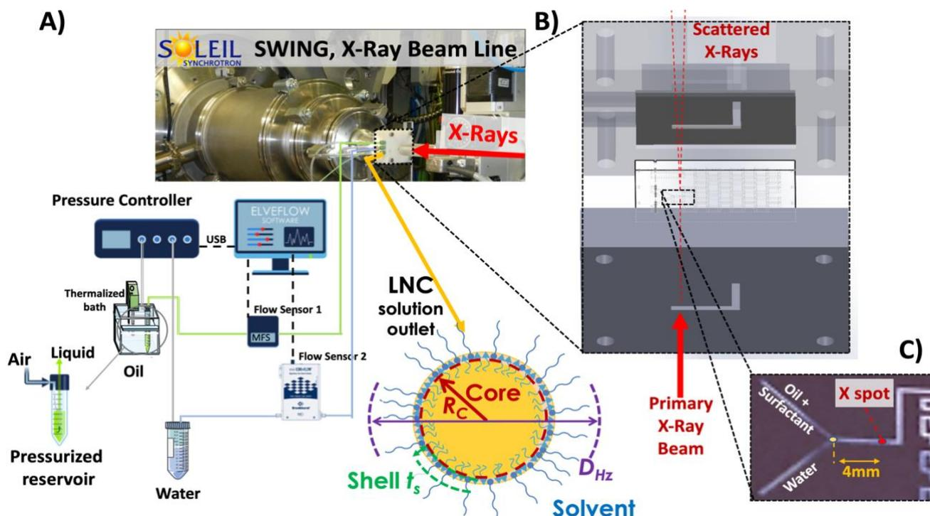
Fig 3: A) Integration of the microfluidic formulation pilot in the SAXS environment at the SOLEIL synchrotron SWING beamline for *in situ* characterization of the LNC structure and their characteristics as the shell thickness ( $t_s$ ), the hydrodynamic diameter ( $D_{Hz}$ ) and the core radius ( $R_c$ ); B) Representation of the microfluidic setup composed of the chip mounted inside the waterblock connector and C) Position of the X-ray beam.
