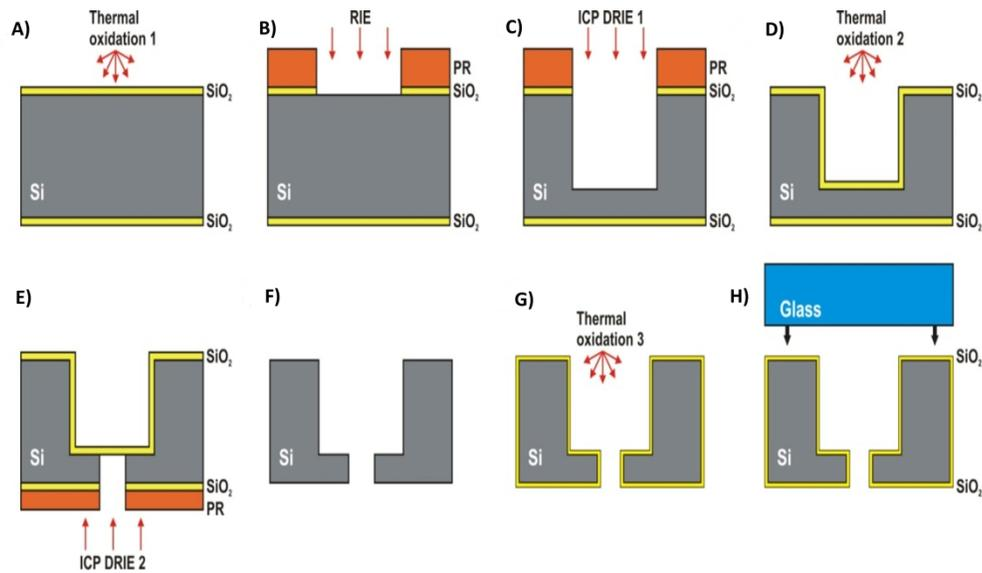
Fig 1: Fabrication process of Si-Glass microfluidic chip, combining the DRIE of silicon and anodic bonding: A) Thermal oxidation of Si, B) photolithography and dry etching of SiO<sub>2</sub> mask, C) DRIE of microchannel, D) stripping of the masks and second thermal oxidation, E) back-side DRIE of via-holes, F) stripping of the masks, G) thermal oxidation (Si surface passivation), and H) anodic bonding to glass lid.
