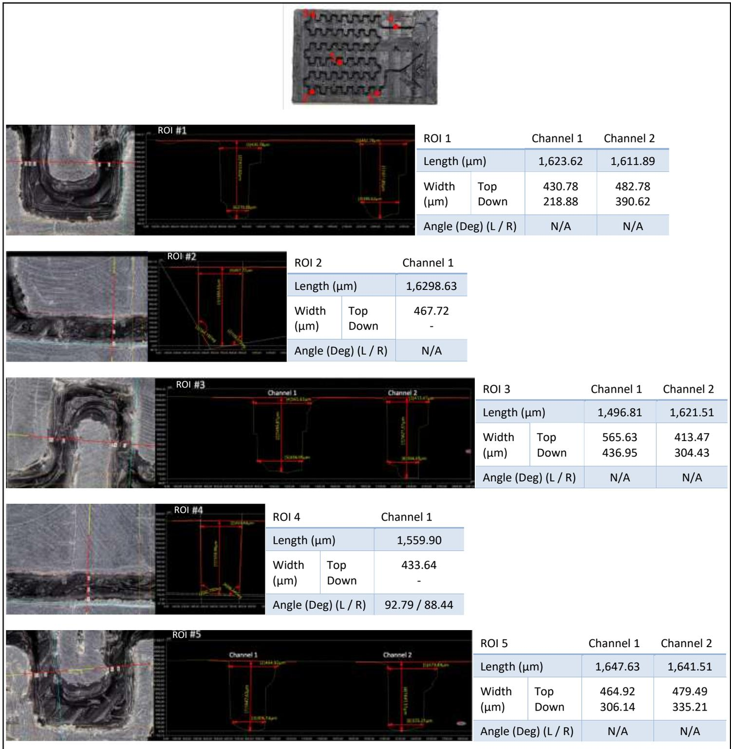
Figure S4-3: Digital microscopy observations of the ABS chip: whole chip (including the localization of the 5 ROI) and zoom on each of the ROI, completed with the software measurement windows and tables with the obtained values.
