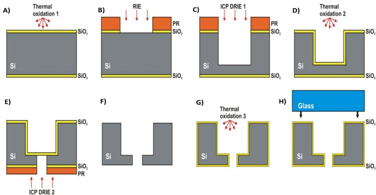
Fig 1: Fabrication process of Si-Glass microfluidic chip, combining the DRIE of silicon and anodic bonding: A) Thermal oxidation of Si, B) photolithography and dry etching of SiO<sub>2</sub> mask, C) DRIE of microchannel, D) stripping of the masks and second thermal oxidation, E) back-side DRIE of via-holes, F) stripping of the masks, G) thermal oxidation (Si surface passivation), and H) anodic bonding to glass lid.
