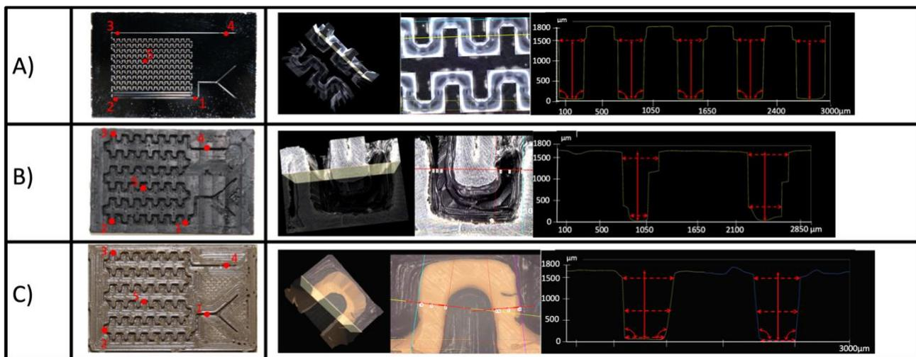
Fig 5: 2D/3D microscopic observations of  $90^\circ$  elbows of A) the Si/Glass chip, B) the ABS chip and C) the PEEK chip. Each Region Of Interest (ROI) are presented for each chip and numbered from 1 to 5. Each chip was observed on the RIO number 5 on this present example.
