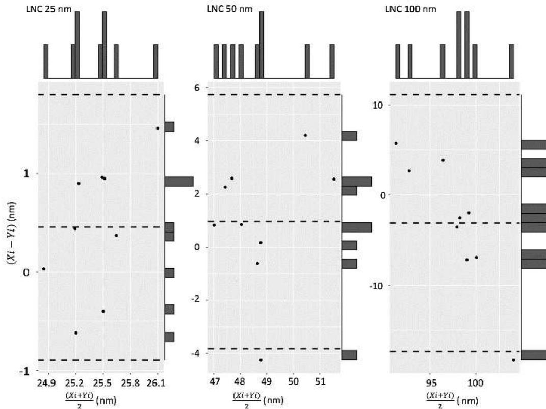
Figure S6-2: Bland-Altman analysis (Si/Glass vs PEEK) for each targeted size (25, 50 and 100 nm). The abscissa axis represents the average size  $(X_i + Y_i)/2$  (with  $X_i$  for Si/Glass size and  $Y_i$  for PEEK size). The ordinate axis represents the size difference  $(X_i - Y_i)$  obtained for a specific condition  $i$ . Bar charts on the right and the top show the occurrence of those values. Upper and lower Dashed lines represent the upper and lower bound of the 95% confidence interval.
