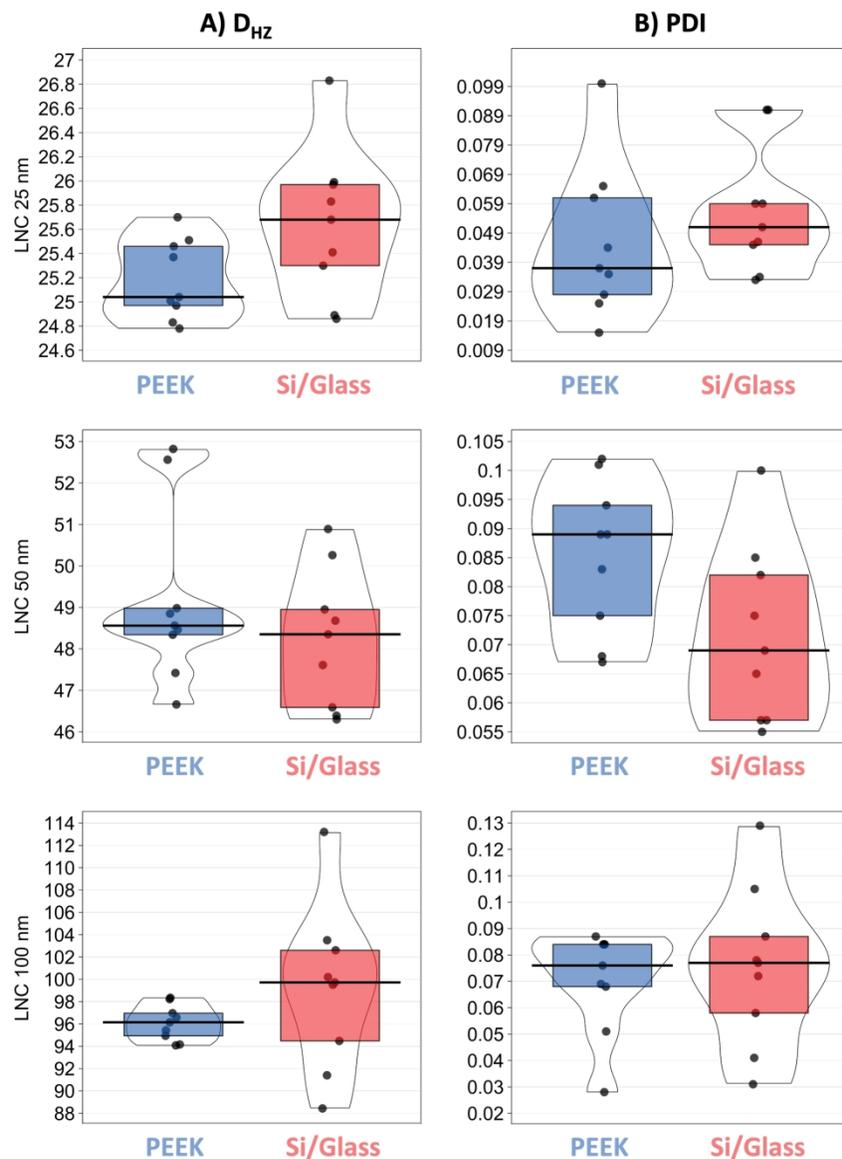
Fig 7: Violin plots of (A)  $D_{HZ}$  and (B) PDI for LNC formulations obtained with PEEK (blue) and Si/Glass (pink) chips. Each boxplot introduces four elements: black points represent raw data, the horizontal black line represents the median, the bean represents a smoothed density and colored rectangles represent the interquartile range.
