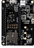
Fig. 2: The Pysense sensor used in this paper’s experiments.
