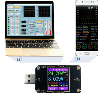
Fig. 3: The energy measurement device used to estimate the current consumption.
