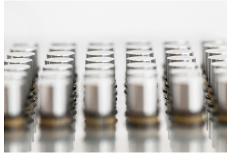
Figure 2. View of the phononic crystal with the adaptive SMP interface
