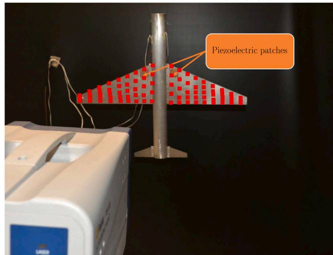
(a) Airplane model equipped with a metabsorber - Structure of the different metabsorber configurations NTMD1/2/3/6/9/18
