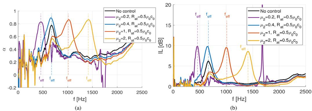
**Fig. 9.** Effect of the variation of the parameters of the control law ( $\mu_1 = 0.4, \mu_2 = [0.2, 0.4, 1, 2]$ ) and target resistance ( $R_{at} = 0.5\rho_0c_0$ ): a) Absorption coefficient ( $\alpha$ ), b) Insertion loss (IL).
