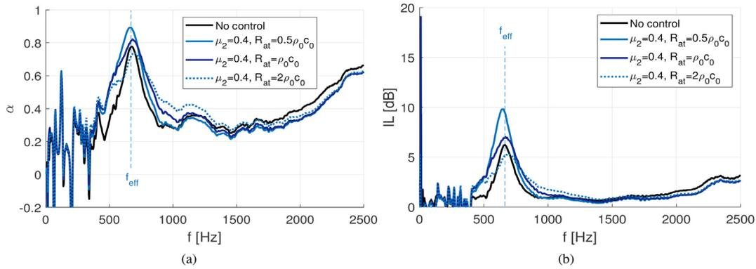
**Fig. 8.** Effect of the variation of the target resistance ( $R_{at} = [0.5\rho_0c_0, \rho_0c_0, 2\rho_0c_0]$ ) and control law parameters ( $\mu_1 = \mu_2 = 0.4$ ): a) Absorption coefficient ( $\alpha$ ), b) Insertion loss (IL).
