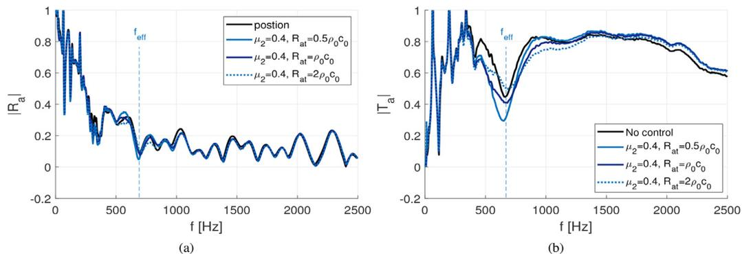
Fig. 7. Effect of the variation of the target resistance ( $R_{at} = [0.5\rho_0 c_0, \rho_0 c_0, 2\rho_0 c_0]$ ) and control law parameters ( $\mu_1 = \mu_2 = 0.4$ ): a) Reflexion coefficient ( $|R_a|$ ), b) Transmission coefficient ( $|T_a|$ ).
