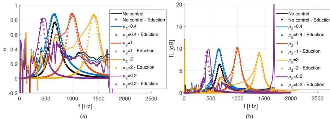
**Fig. 16.** Education - Variation of the parameters of the control law ( $\mu_1 = 0.4, \mu_2 = [0.2, 0.4, 1, 2]$ ), Target resistance ( $R_{at} = 0.5\rho_0c_0$ ): a) Absorption coefficient ( $\alpha$ ), b) Insertion loss (IL).
