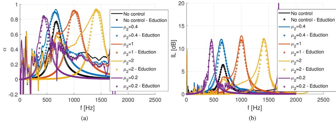
Fig. 17. Education - Variation of the parameters of the control law ( $\mu_1 = 0.4, \mu_2 = [0.2, 0.4, 1, 2]$ ), Transport speed of the advection condition ( $H_{nonloc} : c_a = 0.9c_0$ ), Target resistance ( $R_{at} = 0.5\rho_0c_0$ ): a) Absorption coefficient ( $\alpha$ ), b) Insertion loss (IL).
