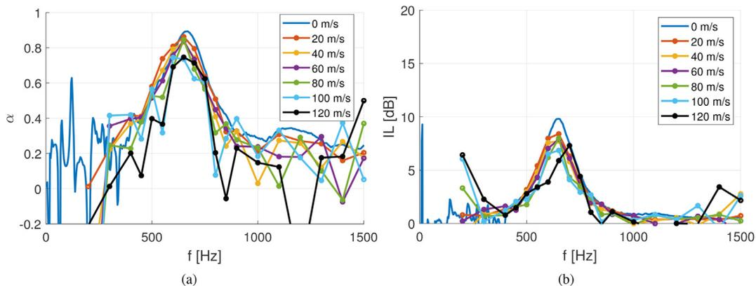
**Fig. 12.** Effect of the variation of flow velocity [20, 40, 60, 80, 100, 120]m/s and control law parameters ( $\mu_1 = \mu_2 = 0.4$ ): a) Absorption coefficient ( $\alpha$ ), b) Insertion loss ( $IL$ ).
