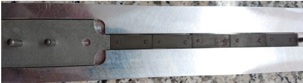
Figure F.1: Partly assembled gMSS in the sample holder prior to the positioning of the upper skin showing the glue points.
