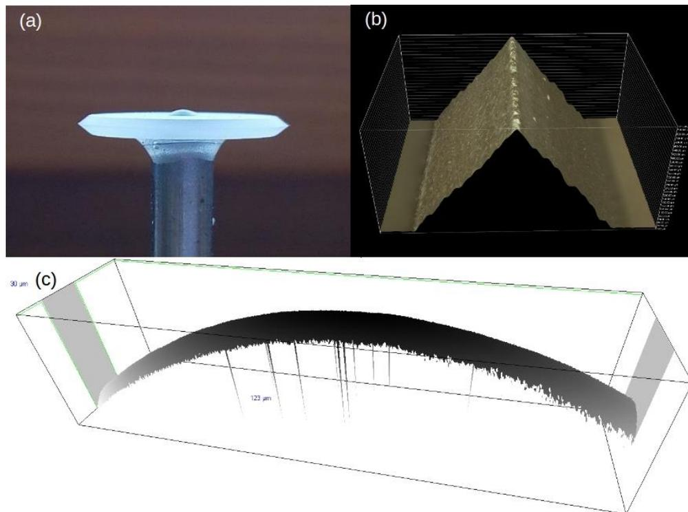
Fig. 2 - Mechanical characterization of preformed disk: (a) photographic image of disk glued to holding stub; (b) microscopic profile reconstruction before polishing; (c) optical profilometry measurement of disk surface after polishing. Measured rugosity after curvature compensation is 4.4 nm over the  $20 \times 123 \mu\text{m}^2$  observation window.
