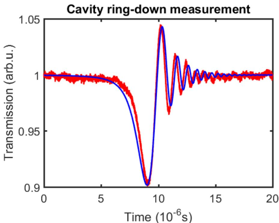
Fig. 3 - Cavity ring-down measurement of disk resonant properties. Red : measured signal, blue : numerical fitting. The intrinsic quality factor used for the fitting curve was  $Q_i = 9.1 \cdot 10^8$ .
