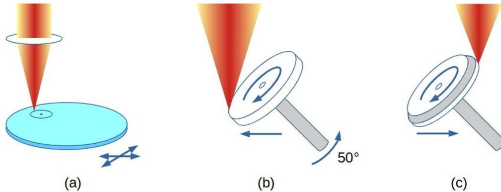
Fig. 1 - Schematic of the machining procedure. (a) Cutting of blank disk from 2" wafer; (b) machining of first bevel angle; (c) machining of second angle. The arrows illustrate the degrees of freedom actively employed during each step. Please note that the beam focusing angle is exaggerated for clarity.
