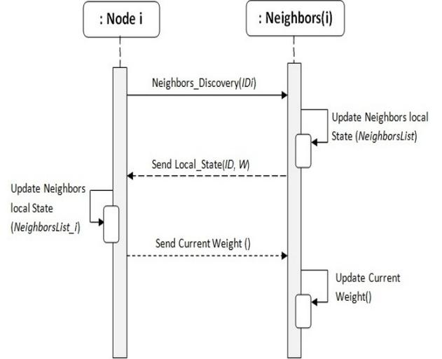
Fig. 2. Sequence diagram of the weight computation procedure
