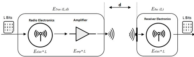
Fig. 5. Radio energy dissipation model
