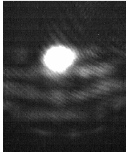
Figure 9. Output of the waveguide, as it is being injected with a 3.39 μm laser
