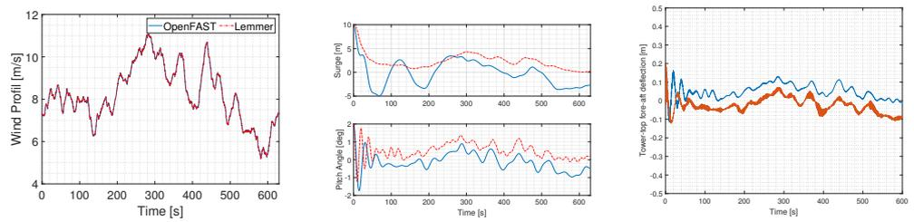
**Figure 5.** Simulation comparison following conditions of [8] with OpenFAST code in blue and Lemmer model in red: wind speed profile (left), surge and pitch translational DOFs (middle) and tower-top fore-aft deflection (right)
