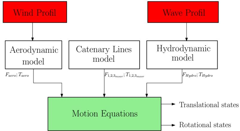
**Figure 1.** Module scheme of the mechanical structure model
