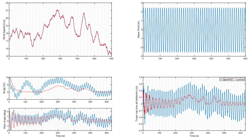
**Figure 6.** Simulation comparison in region 3 with OpenFAST code in blue and Lemmer model in red: wind speed profile (top-left), wave profile (top-right); surge and pitch translational DOFs (bottom-left) and tower-top fore-aft deflection (bottom-right)
