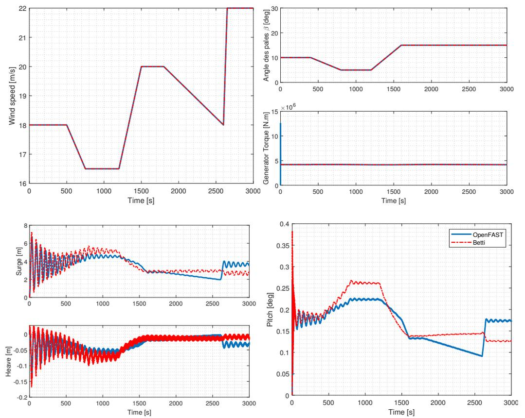
**Figure 4.** Simulation comparison following [4] conditions with OpenFAST code in blue and Betti model in red: wind speed profile (top-left), generator torque and blade pitch angle control inputs (top-right), surge and heave translational DOFs (bottom-left) and pitch angular DOF (bottom-right)
