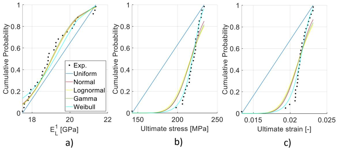
Figure 4. Plot of the experimental dataset and of the cumulative probability functions fitted using usual distribution laws in the case of modulus  $E_L^1$  a), ultimate stress b) and ultimate strain c) for hemp fibre composite.
