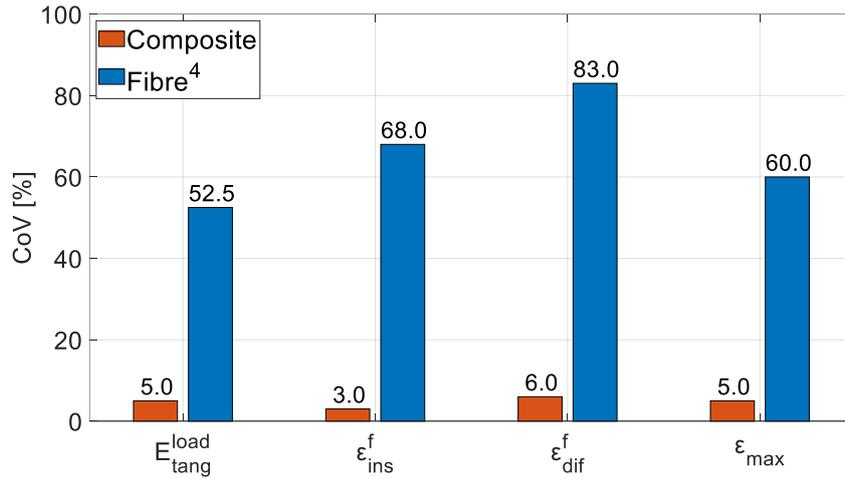
Figure 5. Comparison of the CoV of creep parameters with values from literature at hemp fibre scale (<sup>4</sup> Cisse et al. [17])
