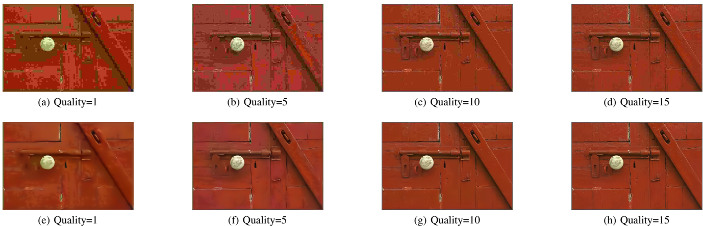
Fig. 10: Corresponding compressed (JPEG) "kodim02" images (a)-(d) and reconstructed ones (e)-(h) by using the proposed model after decompression, respectively versus different image quality, and for the proposed solution without down-scaling operation.
