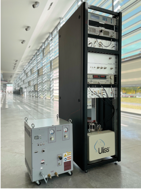
Figure 9. ULISS-2G, the 2nd generation CSO. Notice the He compressor significantly smaller than that of Fig. 8, which takes 3 kW and can be powered from a common 230 V, 16 A outlet.
