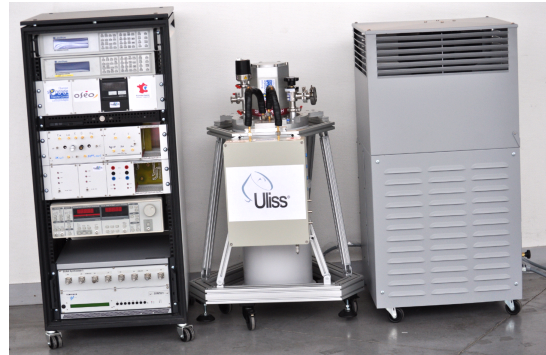
Figure 8. The CSO of 1 st generation: ULISS-1G. Left: 19" rack including the electronic and temperature servos, the frequency synthesis; middle: the cryostat with the sustaining electronics (box in the front); right: air-cooled He compressor. This unit was designed to be transported in a small van to be tested in different sites around Europe. At home, the compressor is replaced with a water-cooled unit.
