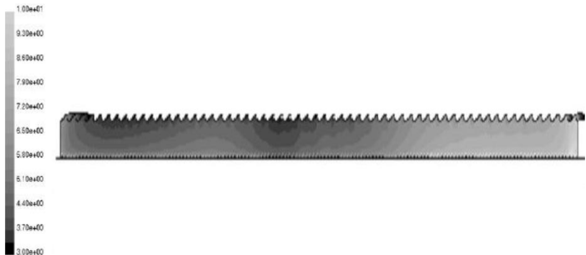
Fig.10 Carbon dioxide dispersion in a 60 span Venlo-type glasshouse with crops (after Reichrath et al., 2001).
