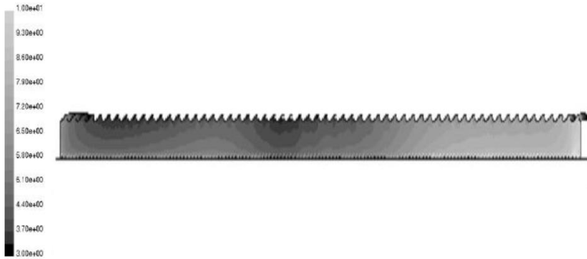
Fig.10 Carbon dioxide dispersion in a 60 span Venlo-type glasshouse with crops (after Reichrath et al., 2001).
