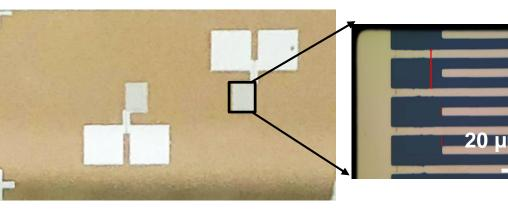
A lithium niobate acoustic sensor was elaborated for specific biodetection.
