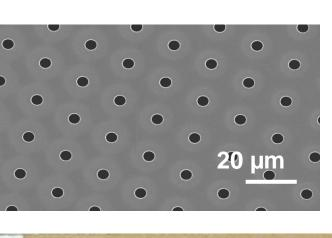
A micro-processed porous membrane was developed for a controlled separation of the microchip chambers.
