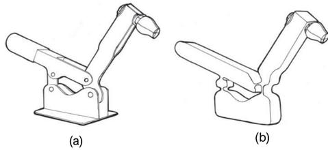
Fig. 2. Mechanisms, (a) rigid-body mechanism of a hold-down clamp (18 parts), (b) compliant hold-down clamp concept (1 part). [51]
