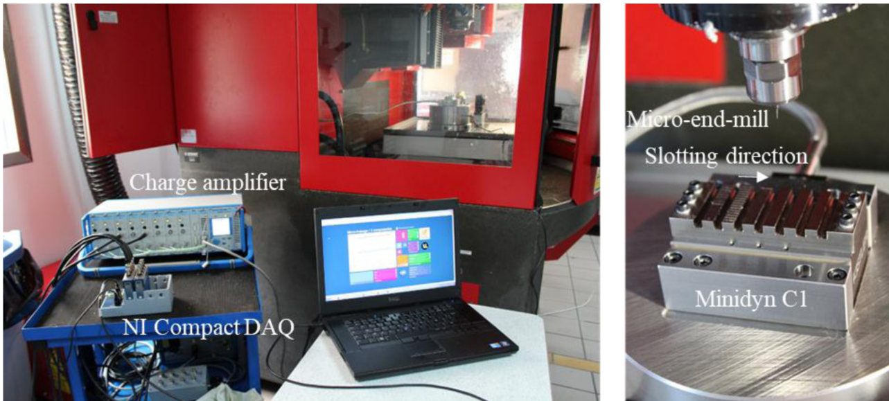
Fig. 7. The experimental configuration for the micro-milling tests.
