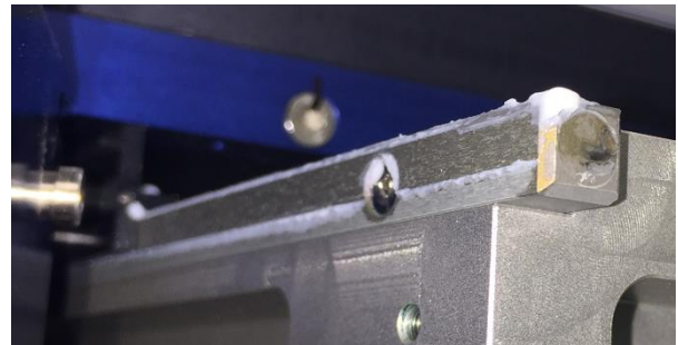
Figure 18 Satellite dummy rail after ejection test : no fretting marks were observed
