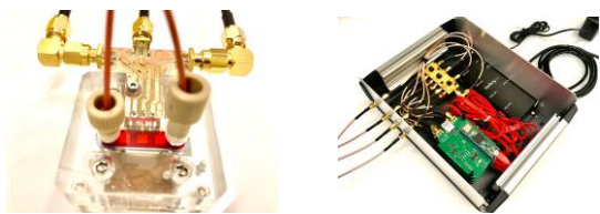
Figure 4: (left) PMMA microfluidic chamber with the 3 sensing units chip and electric readout circuit (right) 3 channel modular electronic for impedance measurement
